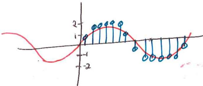
If we sample a signal ranging from 0 to 4 volts with quantized bins of 0.5 volts, we have 8 amplitude levels: 0.5, 1, 1.5, 2, 2.5, 3, 3.5, + 4 volts
